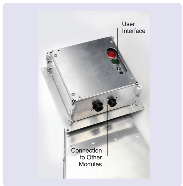
FIGURE 7 The module's nonmoving part. The user interface has two buttons and two LEDs indicating the status of the system. Cables running along the cube structure (not shown) connect the nonmoving parts and allow both the exchange of data and the synchronization of the power circuits. The inertial measurement unit observing the cube motion sits inside the nonmoving part (not shown).
